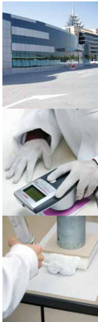
WACKER laboratory in Dubai: installation foam is injected into a test profile to test the post-swelling properties.
