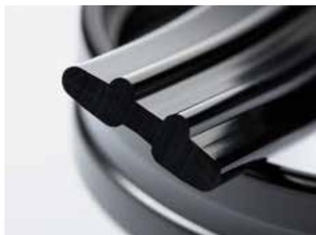
ELASTOSIL® R 771 is currently available in Shore A hardnesses of 60 and 70, and can be compression molded using all conventional processes, extruded or calendered.
