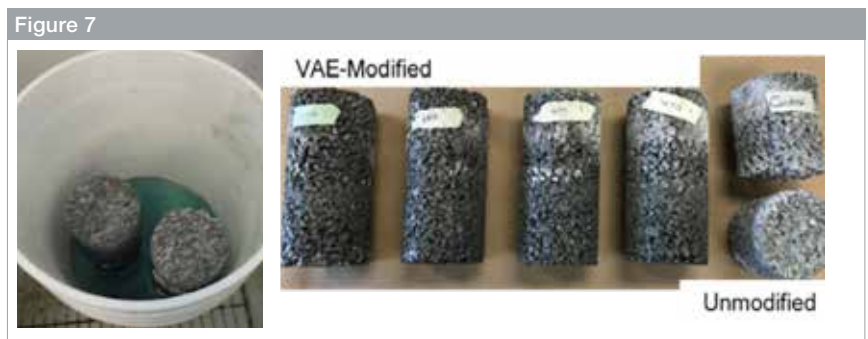
Figure 7 Left: Resistance to deicing salts' test Right: Samples after 35 cycles.
