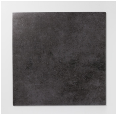
Reference tile used in tests according to EN 14411: unglazed porcelain fully vitrified, Group BI a , E b ≤ 0.5%
