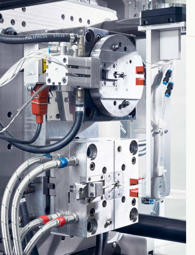
This sort of equipment is used to process liquid silicone rubber at Trelleborg's Stein am Rhein site - under strictly controlled cleanroom conditions.
