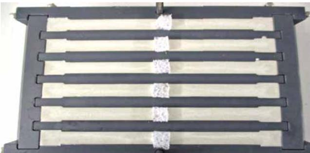
Figure 5a on the left: Central splitting of the test piece with the PE foam divider. Figure 5b on the right: Mold A (6a) filled with fine printing concrete.
