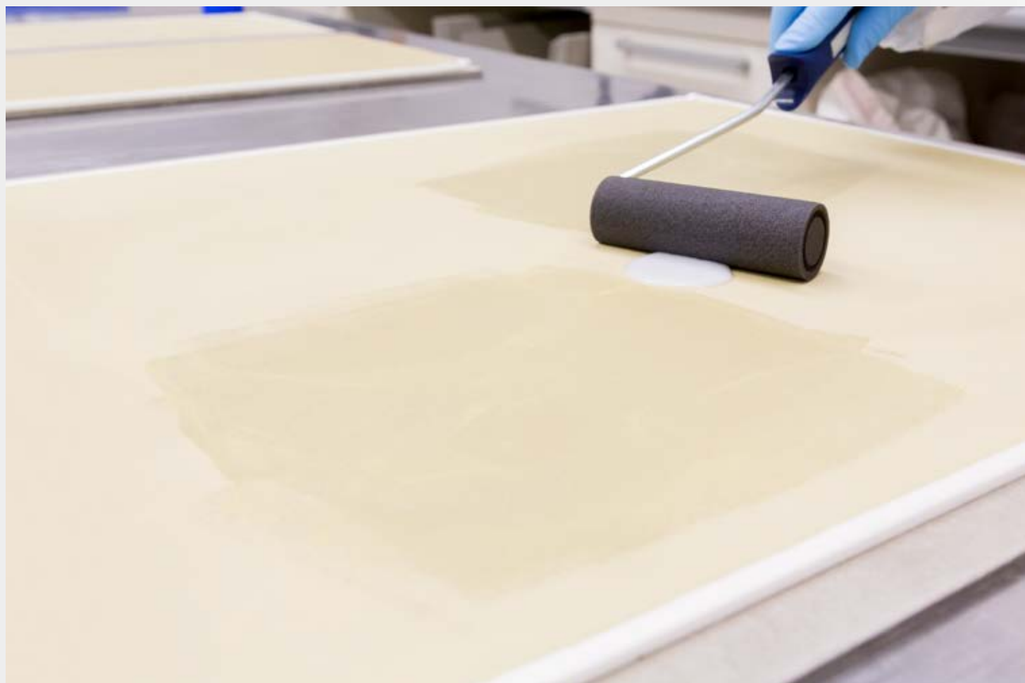
The dispersion can be applied to mineral surfaces in diluted or undiluted form, in line with the specific requirements.
