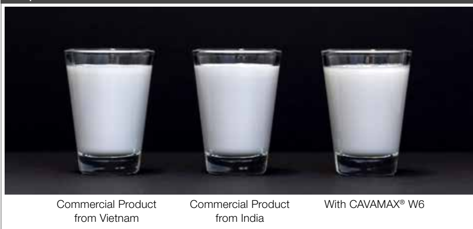
Different coconut milk powder samples were reconstituted in water (20% w/w). The picture was taken after one hour.
