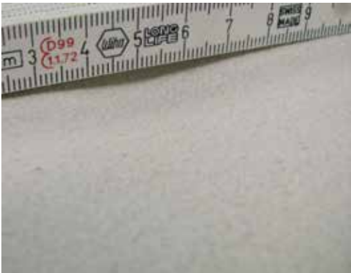
Hard body impact test with 6 joules at 23 °C with 4% VINNAPAS® 5044 N
