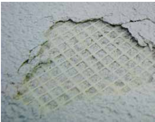
Hard body impact test with 3 joules at 23 °C without polymer modification
