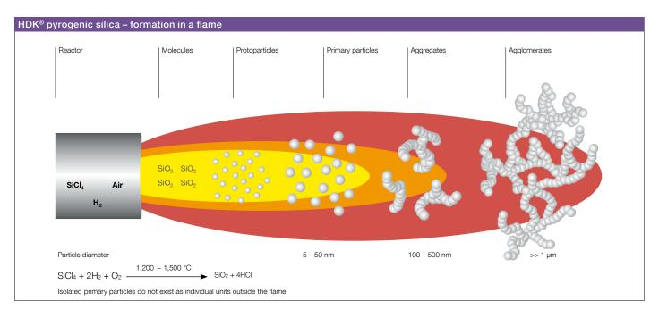
HDK® is produced at multiple sites by an integrated, efficient and environmentally compatible process that saves energy and raw materials.
