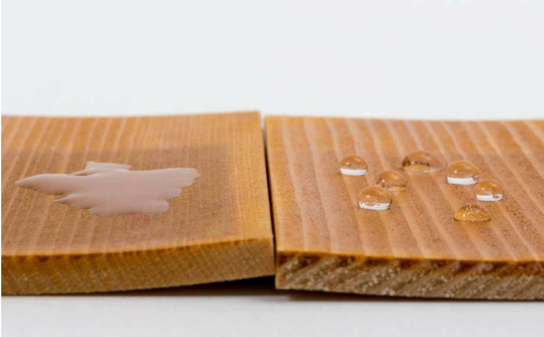
Beading effect after 1,000 h QUV Left: untreated Right: treated with SILRES® WH
