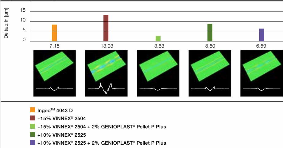
Scratch depth, determined by confocal microscopy including PLA Ingeo™ 4043 D unfilled and compounds with Vinnex® 2504 (polyvinyl acetate/ethylene) plus Genioplast® Pellet P (silicone) or Vinnex® 2525 (polyvinyl acetate) and Genioplast® Pellet P (silicone).
