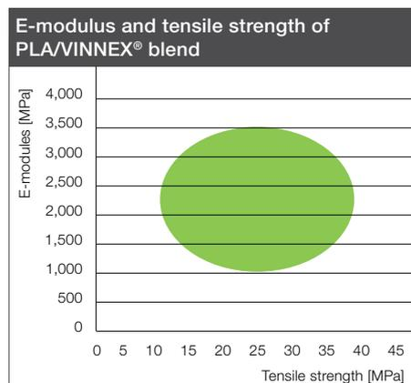
Achievable mechanical properties with PLA/TPS/VINNEX<sup>®</sup> blends for injection molding and thermoforming.
