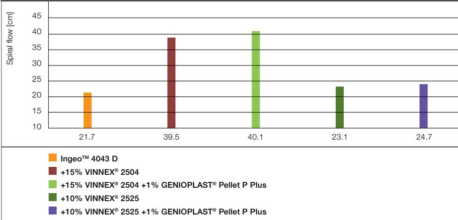
Spiral flow detected with PLA Ingeo™ 4043 D unfilled, and compounds with Vinnex® 2504 (polyvinyl acetate/ethylene) and Genioplast® Pellet P (silicone) or Vinnex® 2525 (polyvinyl acetate) and Genioplast® Pellet P (silicone).
