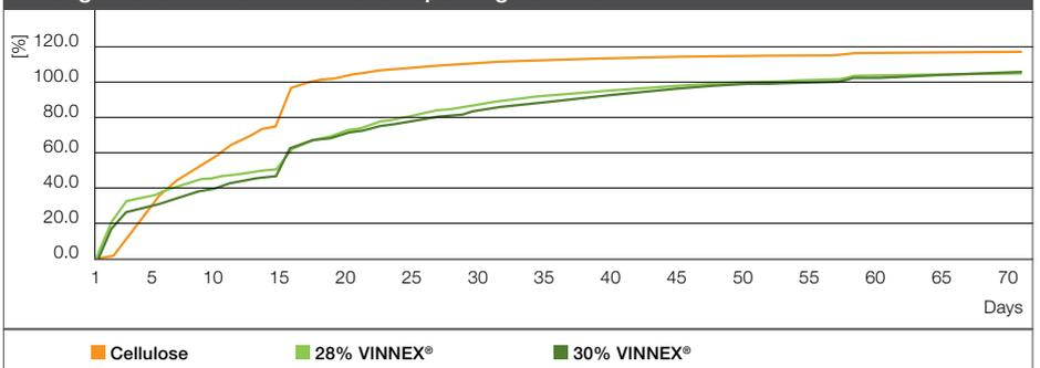
Biodegradation of TPS/PLA/VINNEX® blends under industrial composting conditions (ISO 14855 of EN 13432). On a relative basis with cellulose as the reference substrate, values of 90.0% and 90.1% were calculated. As such, the 90% biodegradability criterion was reached in 65 days both on an absolute and on a relative basis.
