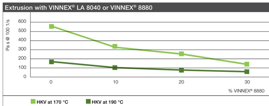
In 3D printing, VINNEX® LA products reduce melt viscosity and increase the flow rate of PLA as shown in the figure above.
