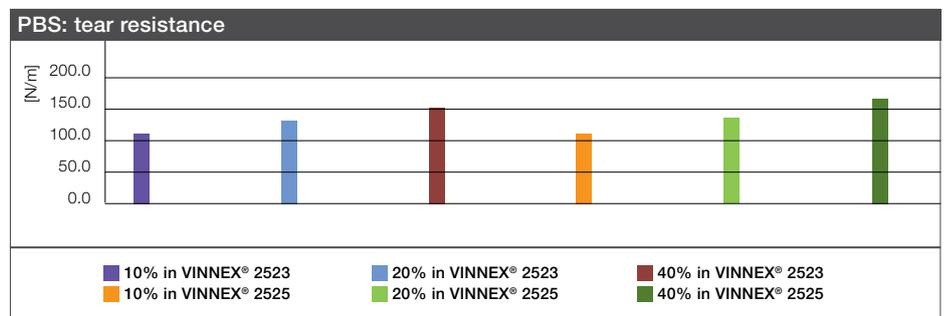
Achievable mechanical properties with PBS/VINNEX<sup>®</sup> resin blends for injection molding and thermoforming.
