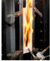
The new dispersion VINNOL® CEN 2752 with a reduced formaldehyde content is particularly suitable for textiles with stringent flame-retardancy requirements. Laboratory tests show whether textiles pass the relevant flame test (example left) or are readily flammable (example right).
