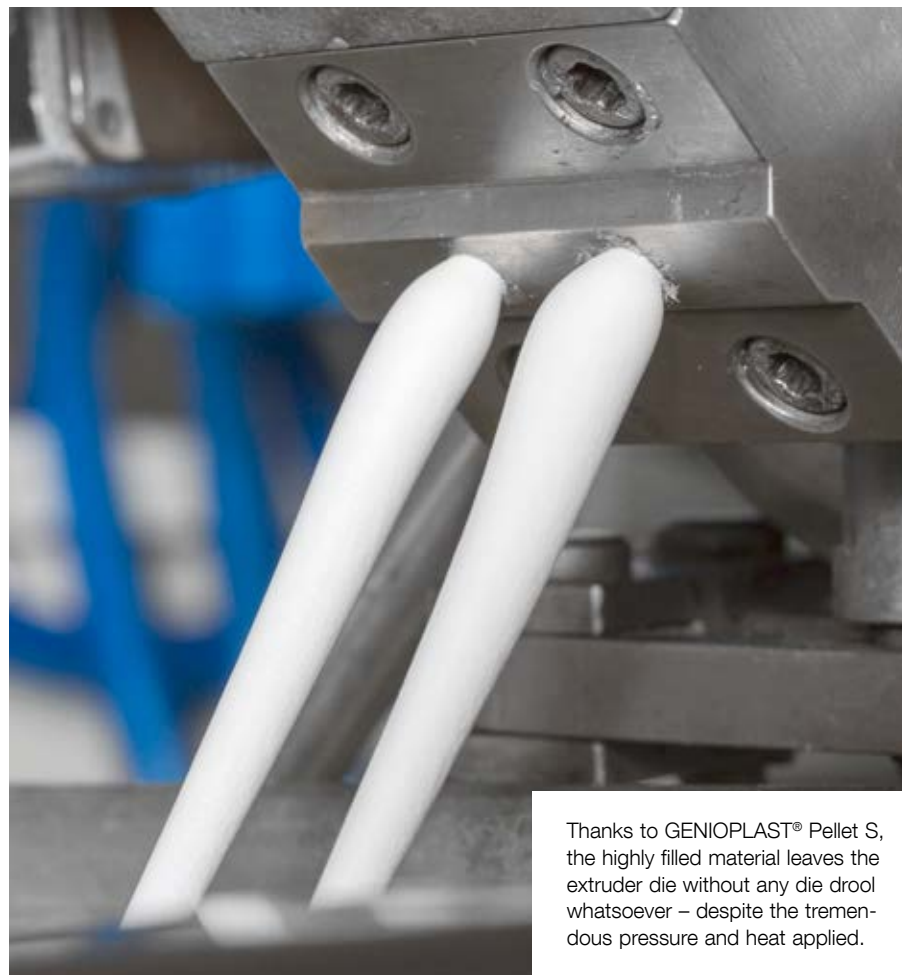
The silicone pellets are poured into a gravimetric dosing station where they are combined with flame-retardant fillers such as aluminum trihydroxide and a thermoplastic polymer such as polyethylene or polypropylene. The materials are compounded to form a homogeneous mass.
