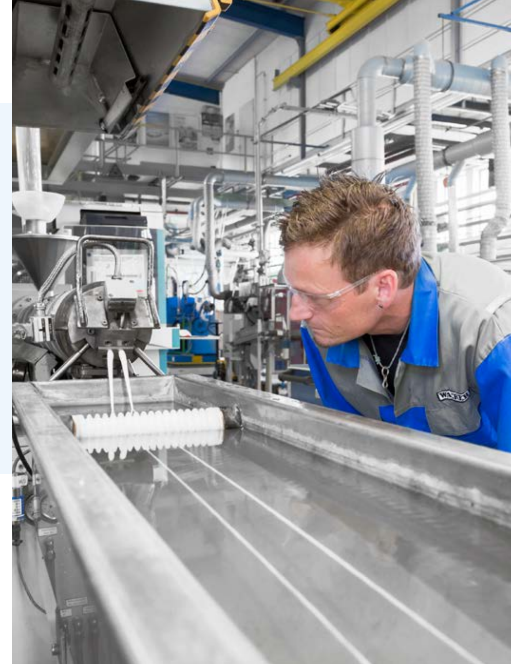
Development engineer Oliver Fuhrmann observes the discharge of molten compound into the water quench.
