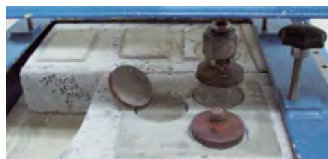
Mortars modified with VINNAPAS® have excellent adhesion: tests show a bond strength of 0.6 N/mm 2 .
