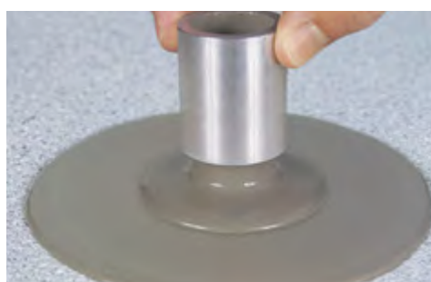
Flow test: the influence of VINNAPAS® dispersible powders measured with an ABS ring.
