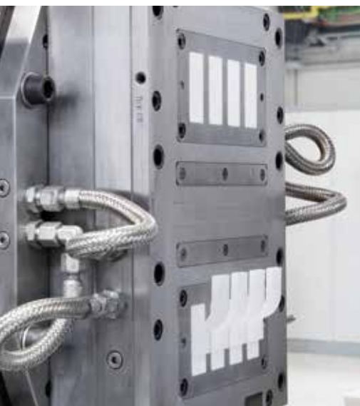
Injection molding machine for 2K materials
