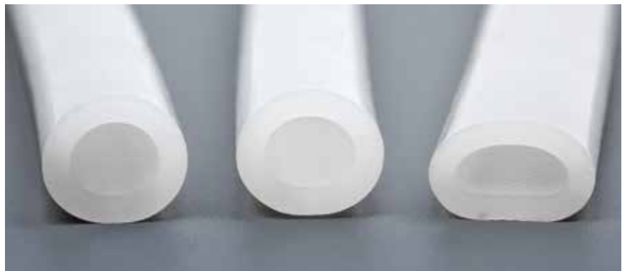
Fluctuations in the extrudate geometry
