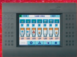
Hopper loader status
