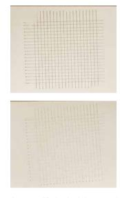
An unmodified polyethylene panel evidences significant scratches after the scratch test (see top image). Scratch resistance was significantly improved through the addition of GENIOPLAST® PE50S08 (bottom image).
