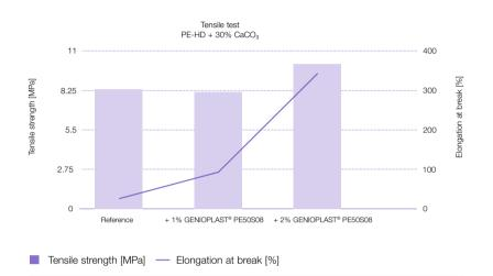
The addition of GENIOPLAST® PE50S08 was positively evaluated in the tensile test. Chalk-filled HDPE evidenced greater tensile strength and a higher elongation at break.
