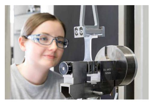
Peel testing stresses samples of multicomponent materials to their breaking point. In samples made of ELASTOSIL<sup>®</sup> LR 3078 and polycarbonate, it was the soft silicone component which consistently tore. The bond between the hard and soft components remained intact.
