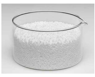
Silicone additives - here as ready-to-use pellets - facilitate the production of workable polyethylene molding compounds and improve the surface properties of the resulting plastic articles.
