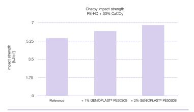
The addition of 2% GENIOPLAST® PE50S08 to chalk-filled high-density polyethylene increased the impact strength measured during Charpy impact tests by a good 20%.
