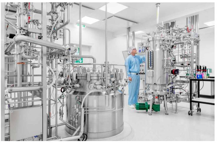
Bacteria at Wacker Biotech in Halle produce pharmaceutical proteins in stainless steel tanks known as fermenters. The site is being expanded into an mRNA competence center, scheduled to start up in 2024 and featuring a new technology.
