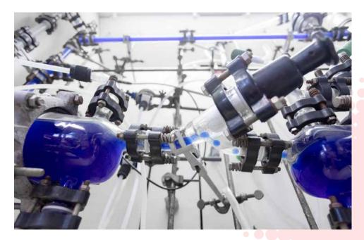
Glass circulating reactor: WACKER has developed a continuous manufacturing process for resin binders at a technical service lab at its Burghausen production site.
