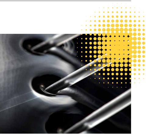
Preliminary stage for the production of blown or cast film: transparent pellet stock is made from a bioplastic and VINNEX® 2526. During this process, the strands pass through a water bath.
