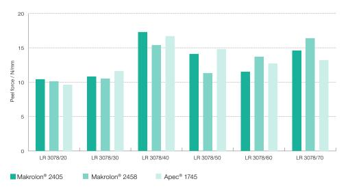
Adhesion was tested by conducting 90° peel tests on multicomponent specimens made from all the grades in the ELASTOSIL® LR 3078 series and three commercial polycarbonate grades. Peel-force values higher than 10 newtons per millimeter signify excellent adhesion.
