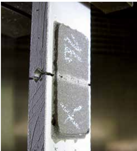
Flexible waterproofing membranes can bridge cracks caused by movement of the substrate.
