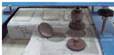
Mortars modified with VINNAPAS® have excellent adhesion: tests show a bond strength of 0.6 N/mm.
