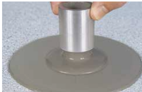
Flow test: The influence of VINNAPAS® L Class powders measured with an ABS ring.
