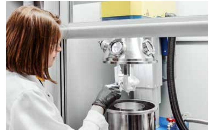
At the technical center in Moscow, a lab assistant mixes a low-modulus sealant, based on silane-modified polyether, with a planetary mixer.
