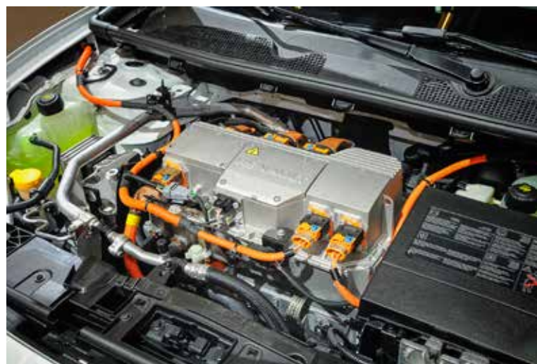
A peek into the engine compartment of a Renault Fluence: this vehicle was equipped with a traction battery that could be replaced at special stations. Time-consuming charging was therefore no longer necessary. The thick orange high-voltage cables are clearly visible under the engine hood.
