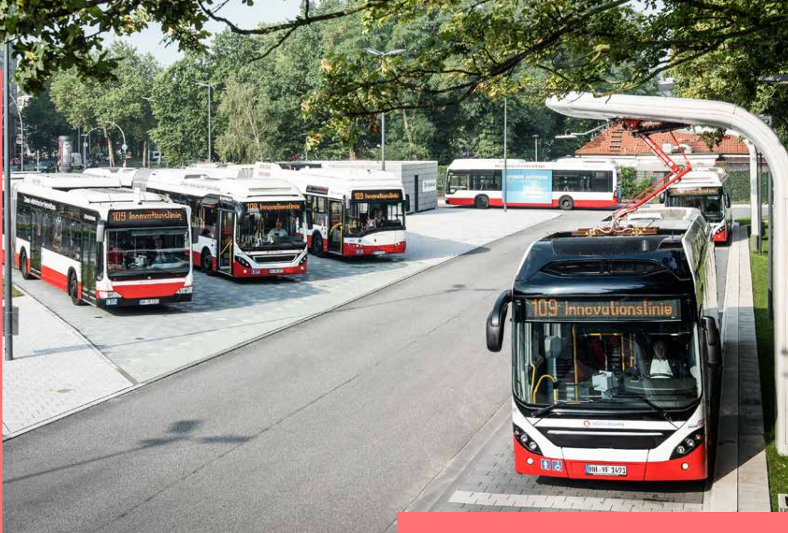
A Volvo hybrid bus operated by the Hamburger Hochbahn public transport company (HHA) at a charging station: HHA wants to convert its entire fleet of approximately 1,000 vehicles from diesel to electric drive over the next few years.
