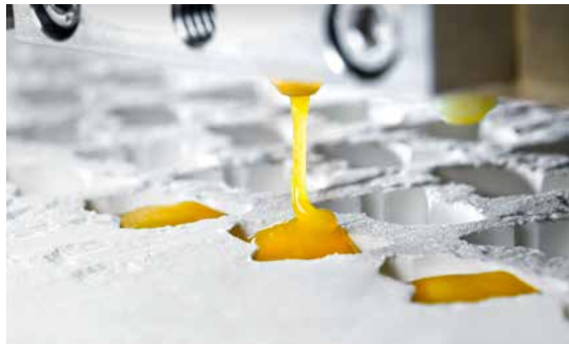
The rheology and viscosity of a mixture can be adjusted so as to prevent undesirable phenomena such as a stringy consistency or entrapped air.
