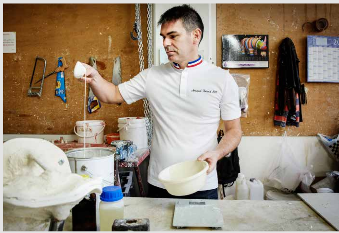
Above The master craftsman, who bears the title of Meilleur ouvrier de France , blends the silicone. He knows the formulation by heart and adjusts it to suit the current room temperature and humidity.
