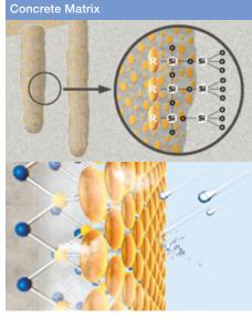
permeability, and long durability, which stems from silanes' high resistance to external influences such as UV radiation, thermal stress, aggressive substances, and microbes. This is due to extremely stable covalent bonds between the silane and the silicate matrix of the pores and capillary walls in the concrete.
