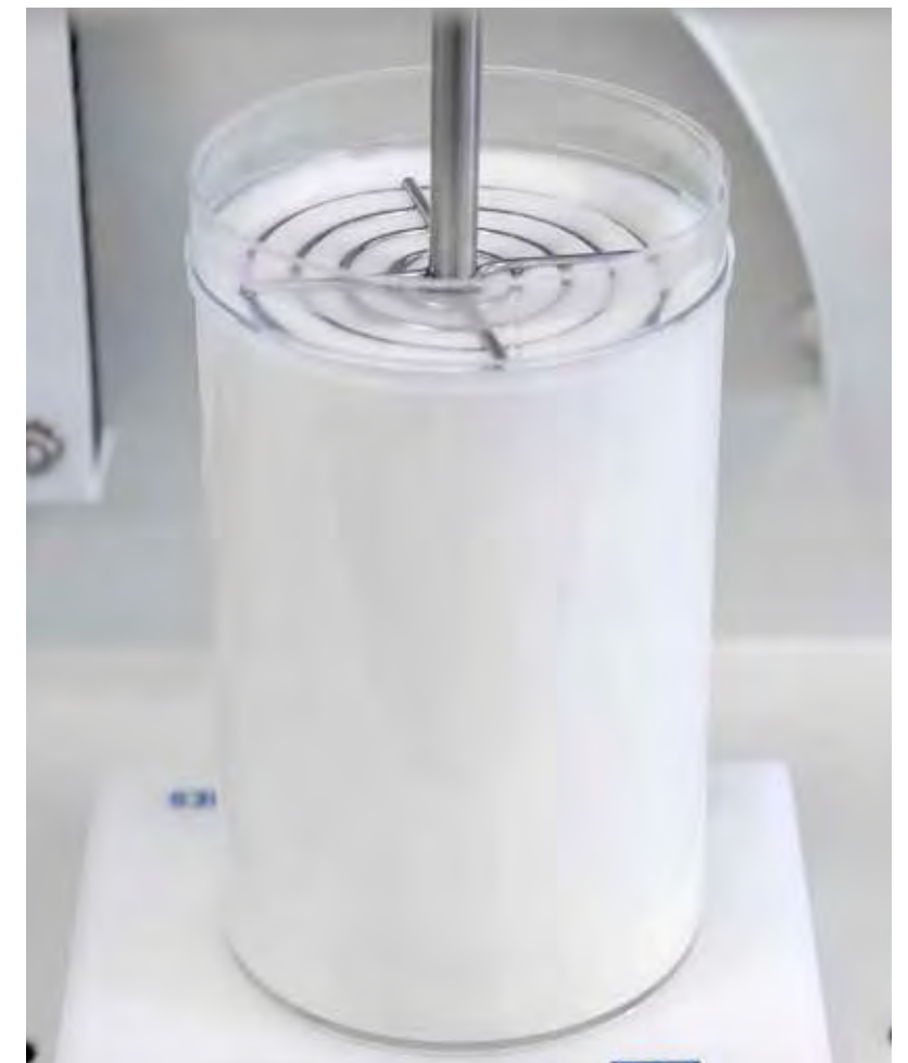
A look inside the food lab in Burghausen: technicians use this test setup to measure foaming capacity.
