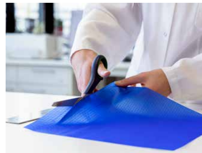
An applications lab employee in Burghausen cuts a piece of ripstop nylon fabric to size so as to measure its tear resistance.
