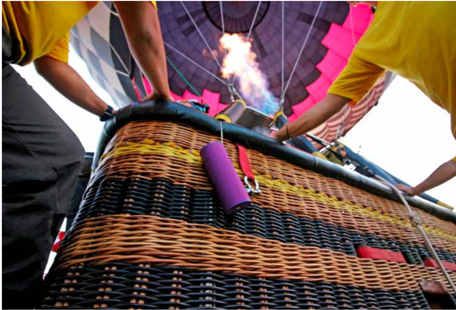
A hot-air balloon before takeoff: the upper half of the envelope is under particularly high thermal stress – as this is where the hot air accumulates – and thus lends itself to being coated with silicone.
