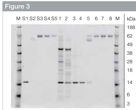
Figure 3: SDS-PAGE image of the purification of pegylated Anticalin®: M - Protein molecular weight marker, S1-S5 standard positive controls: S1 - free Anticalin®, S2 - free PEG, S3-S5 - pegylated Anticalin® in different concentrations. Lanes: 1 - after clarification, 2 - after filtration, 3 - main fraction from capture chromatography, 4 - main fraction from intermediate chromatography, 5 - after pegylation, 6 - main fraction from polishing chromatography, 7 and 8 - final product
