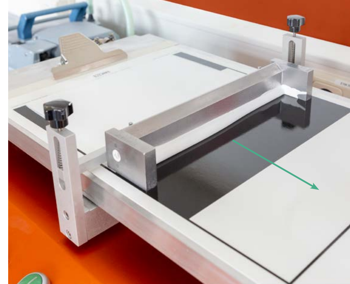
To test its hiding power, the paint is spread evenly over a black substrate. The contrast ratio is then measured.
