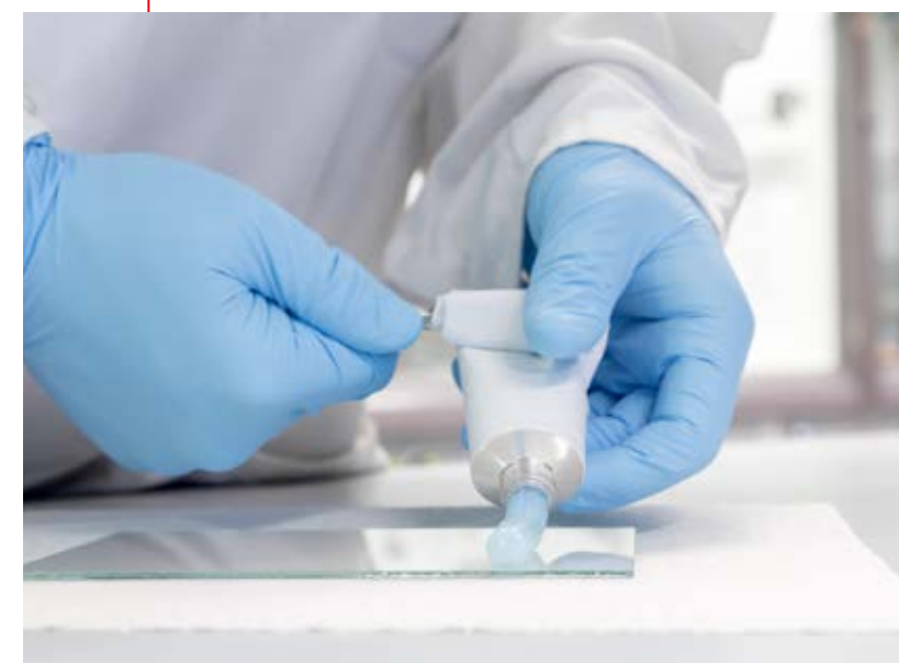
A member of WACKER's technical support team presses an epoxy resin adhesive onto a pane of glass. The adhesive sample at the bottom right has been formulated with HDK® H21 and therefore exhibits much better sag resistance – it does not run, unlike its counterpart.
