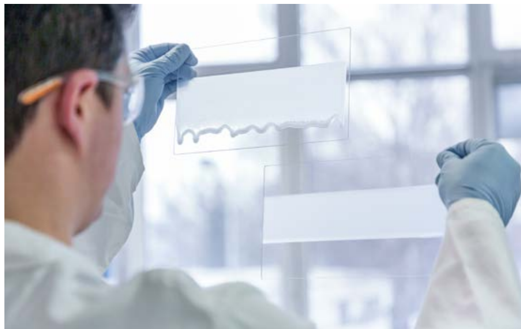
An epoxy resin rendered thixotropic with HDK® H21 is applied to an inclined pane of glass: the polar adhesive component containing HDK® does not run and the layer exhibits sag resistance.
