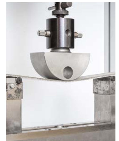
The deformability of tile adhesives is tested to EN 12004-2 at WACKER's applications laboratory.
