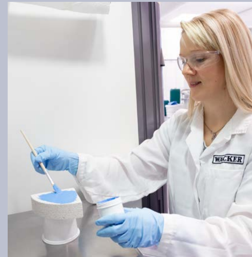
Paint containing VINNAPAS® EP 3560 is applied to a cinder block test piece at WACKER’s applications laboratory.
