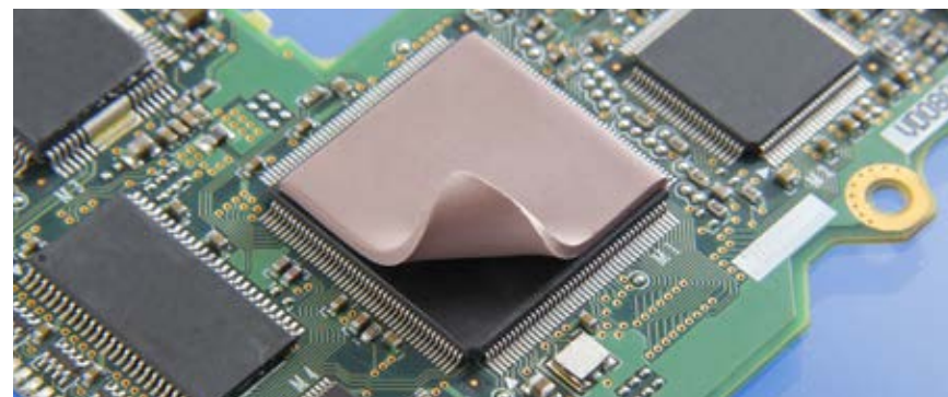
SARCON® thermal gap filler pads from Fuji Polymer Industries are highly conformable, thermally conductive gels in versatile sheet form. They adhere to all shapes and sizes of components, even when they feature protrusions or recessed surfaces.
