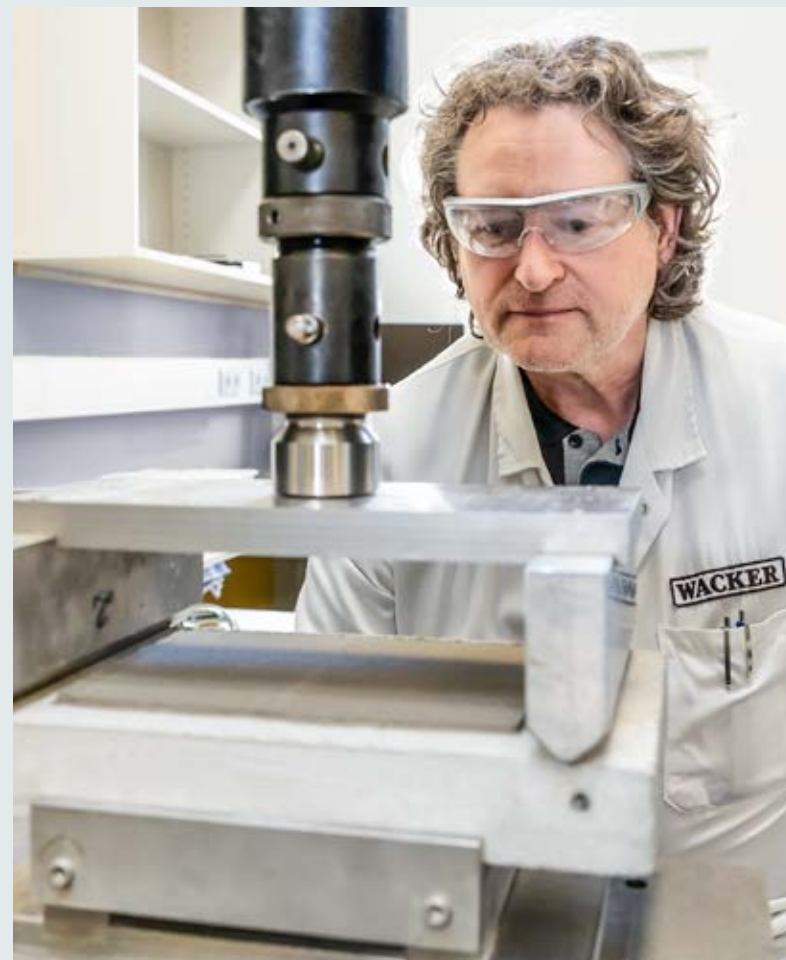
A lab technician tests the deflection of the concrete test piece as per EN 1062-7. This standard stipulates that cracks must not exceed a width of 0.4 millimeters.
