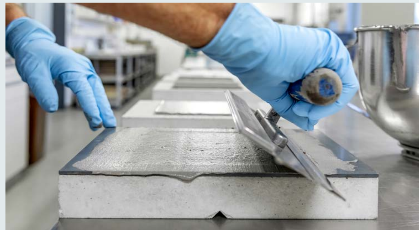
To perform the crack-bridging test as per EN 1062-7, the waterproofing membrane is spread to a defined film thickness.
