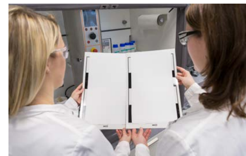
When directly compared with conventional wall paint, the good hiding power of paint modified with VINNECO® CT 7030 is confirmed.
