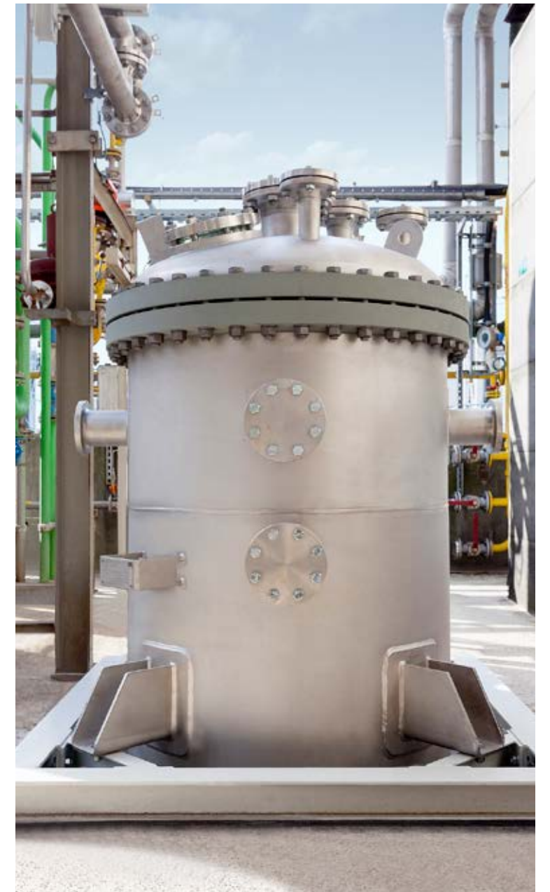
The new IPA reactor is part of the integrated ketene production system at WACKER’s site in Burghausen, where acetic acid is converted into ketene, isopropenyl acetate and acetylacetone in various steps.
