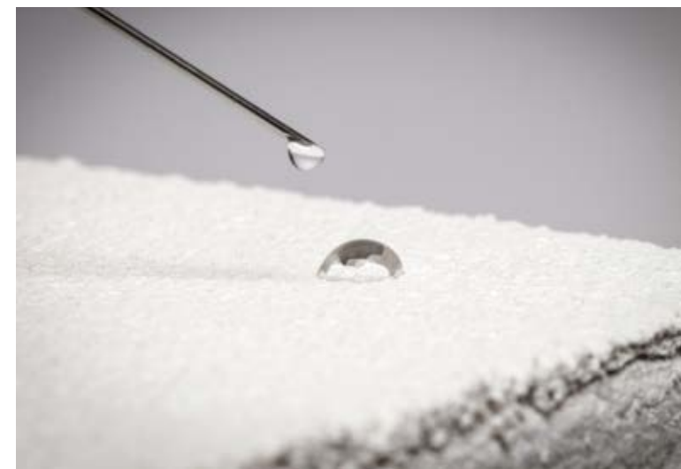
Finishing or filling plasters modified with water-repellent VINNAPAS® dispersible polymer powders improve weathering resistance and the longevity of buildings.
