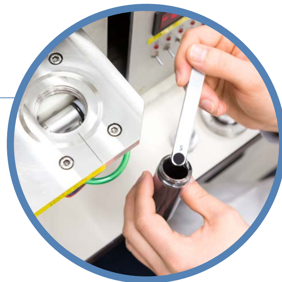
Magnetic dry toner is metered onto a rotating roller, charged, and artificially aged to simulate a certain number of copies. The instrumentation determines the charge transferred to the toner.
