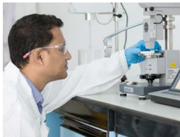
The WACKER laboratory for silicone elastomers in Dubai: an employee performs a Shore hardness test.
