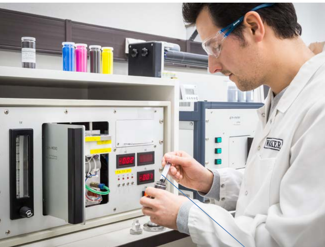
Investigating the chargeability and flowability of a dry toner in the lab.
