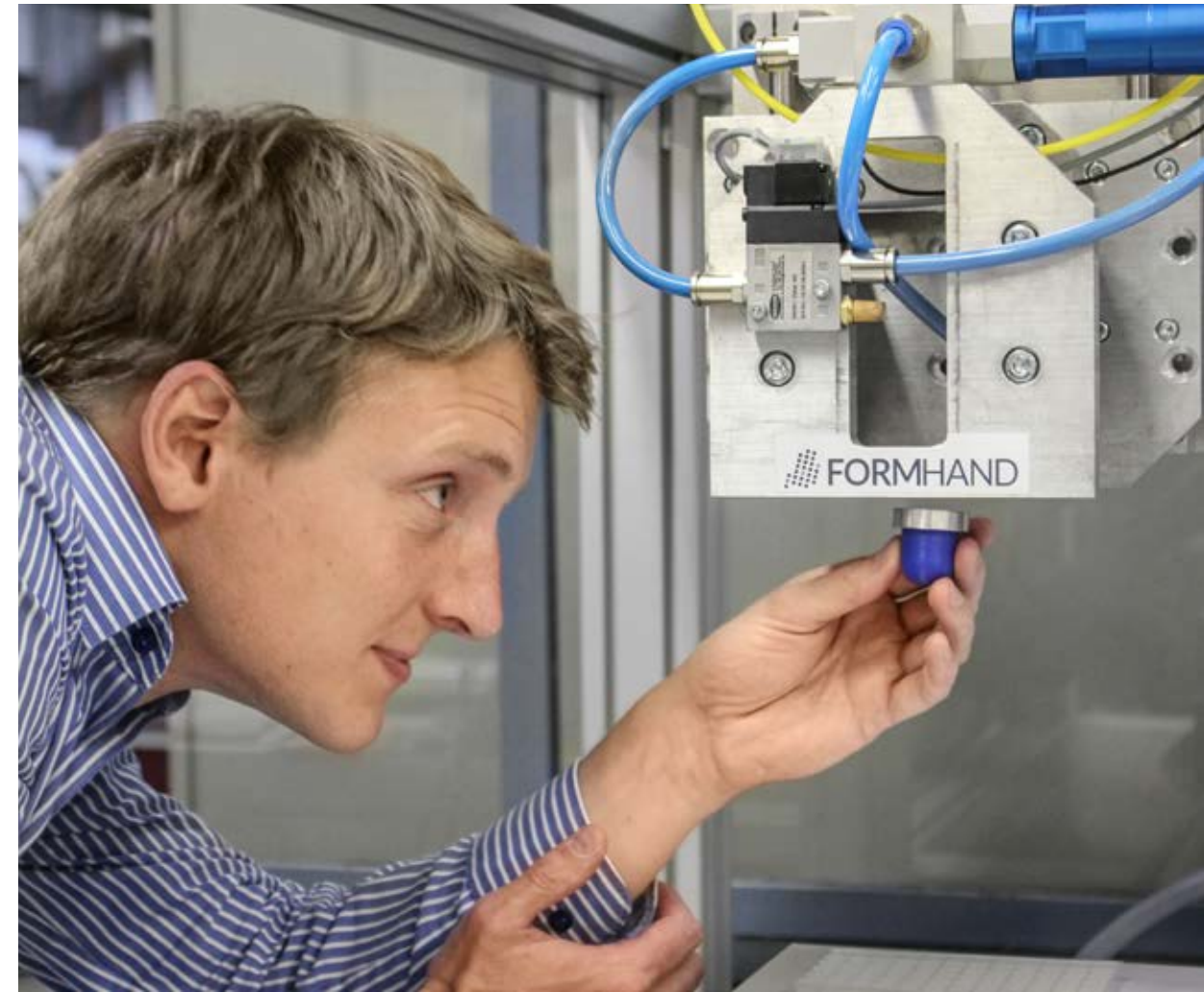
Holger Kunz, founder of startup Formhand, takes the new, extra-small silicone cap made by the 3D printer and fits it on the robot.
