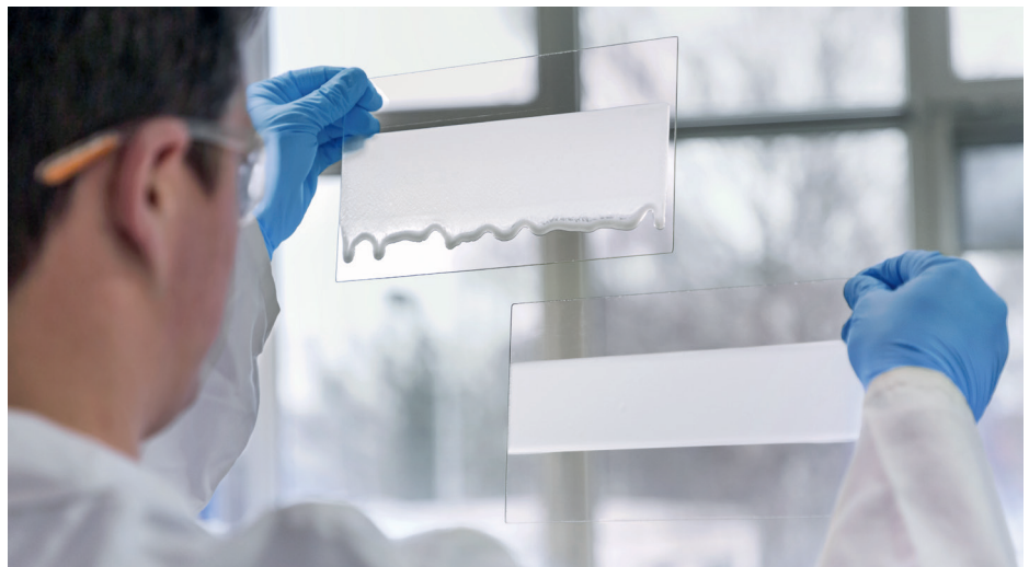
Hydrophobic HDK® grades such as HDK® H18 and HDK® H21 ensure highest sag resistance in epoxy-based adhesives where standard hydrophobic grades fail.
