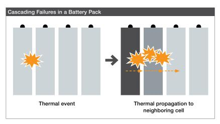
The important safety criterion for batteries is to keep the temperature within the desired working range and preventing cascading failures from one cell to another in a battery pack. A cascading failure is typically accompanied by a sustained fire which further accelerates the battery failure. WACKER offers various silicone solutions aimed at keeping battery temperatures within the optimum range, increasing battery safety in general and, in particular, preventing fire propagation.
