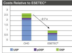
Total costs of single GMP batches relative to ESETEC®. The cost of goods is reduced up to 2.7-fold due to shorter process times, reduced media costs, and viral depletion steps.
