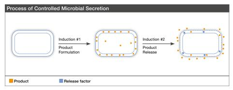
The principle: after a production phase and accumulation of the product in periplasm, the addition of an inductor actively starts the release of the product into the culture broth
