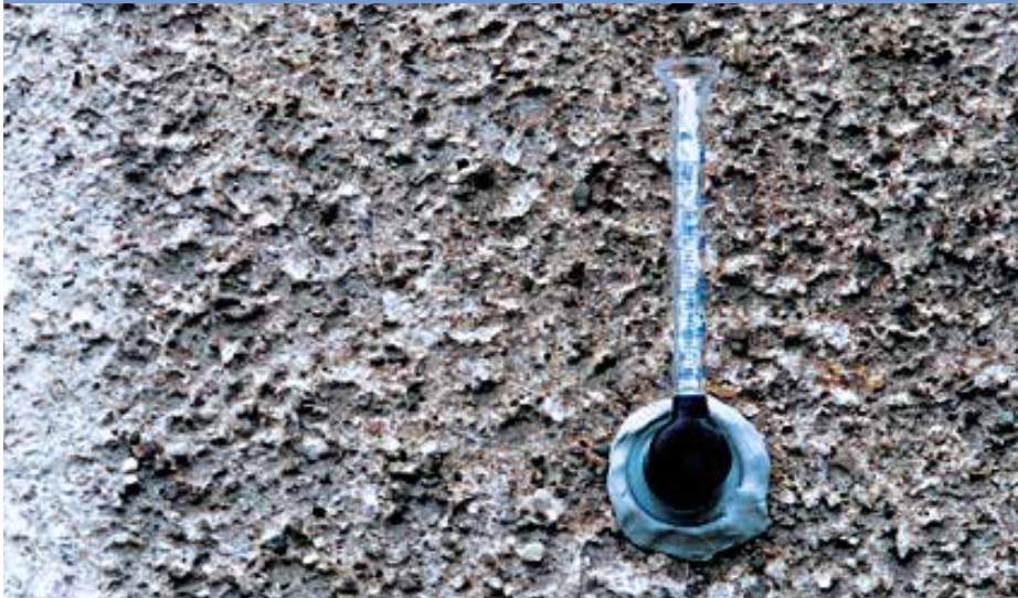
Untreated: water travels very readily into the substrate.
