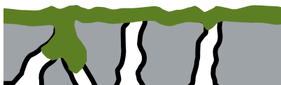
Film-forming systems (coating and impregnation) will not be permeable to water vapor. Damage enables water to penetrate and cause further damage.
