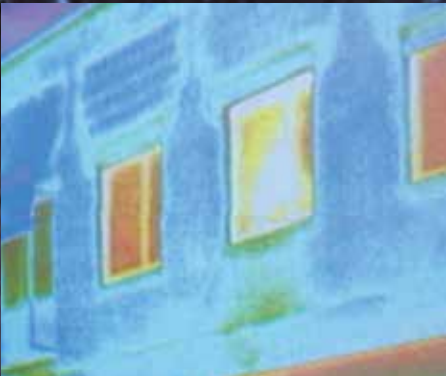
Water reduces the insulation behavior of a facade. A dry facade helps to reduce energy costs.
