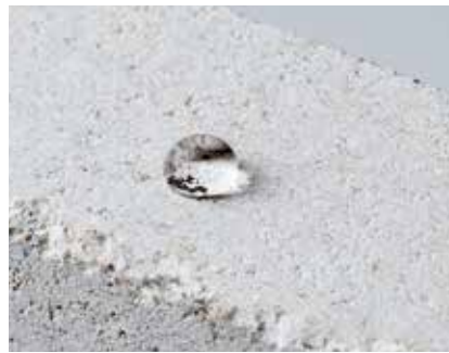
When a hydrophobic impregnation is applied, the water beads off.
