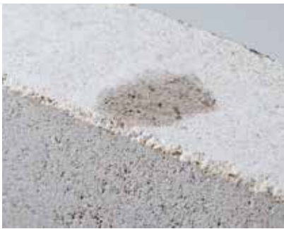
The untreated substrate absorbs water.
