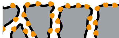
SILRES® BS results in a good penetration depth. It is not film-forming and therefore allows water vapor to escape.
