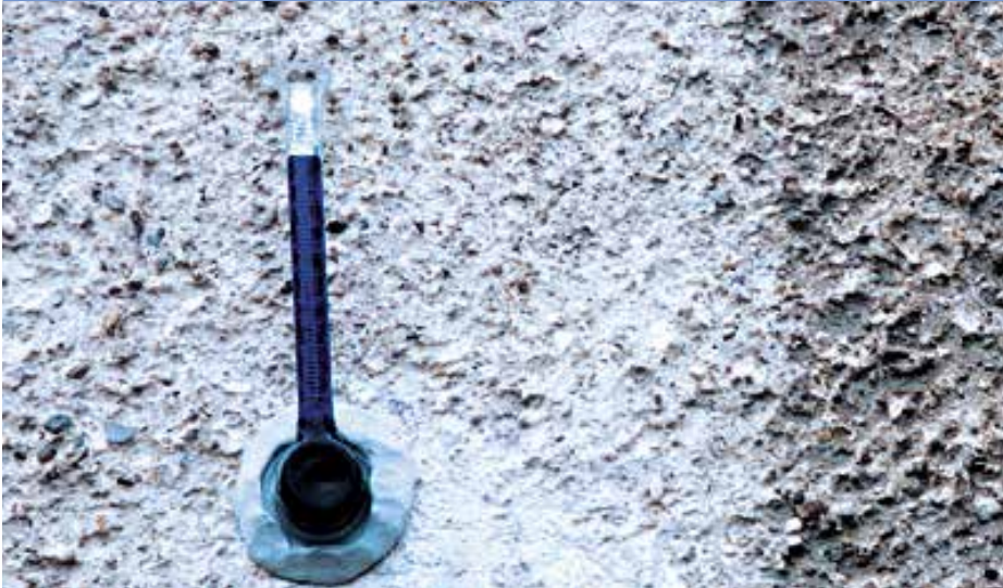
Treated in 1954: even after more than 50 years, water does not penetrate into the substrate.
