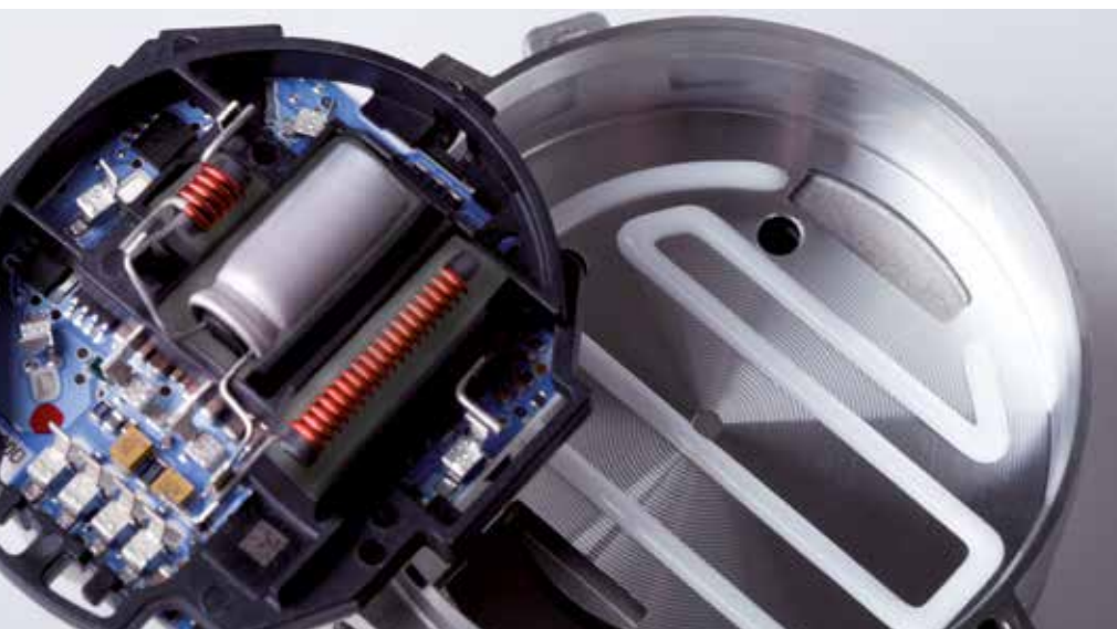
The image depicts the bonding of a ceramic substrate to a die-cast aluminum housing with SEMICOSIL® 971 TC. The LC module is then encapsulated with ELASTOSIL® RT 743 LV-K.
