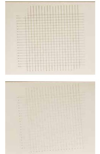
An unmodified polyethylene panel evidences significant scratches after the scratch test (see top image). Scratch resistance was significantly improved through the addition of GENIOPLAST® PE50S08 (bottom image).
