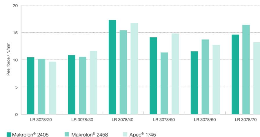
Adhesion was tested by conducting 90° peel tests on multicomponent specimens made from all the grades in the ELASTOSIL® LR 3078 series and three commercial polycarbonate grades. Peel-force values higher than 10 newtons per millimeter signify excellent adhesion.
