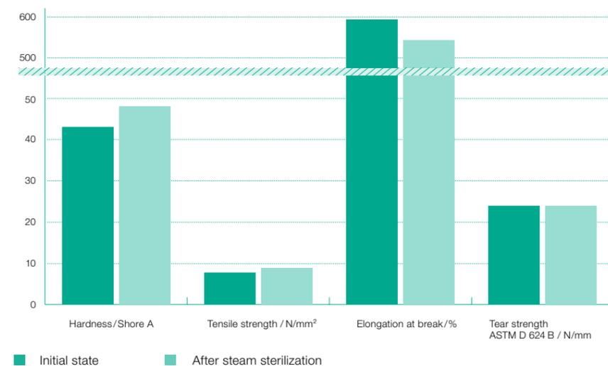
Not even 100 steam sterilization cycles in the lab were able to reduce the mechanical properties of test specimens made with ELASTOSIL® LR 3078. They remain at a consistently high level (ISO 17665 – Aging test as per EN 868-8; 134 °C, 5 min).
