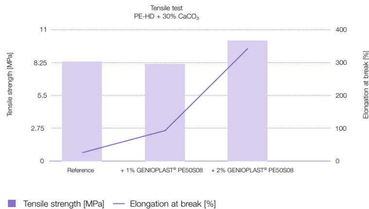
The addition of GENIOPLAST® PE50S08 was positively evaluated in the tensile test. Chalk-filled HDPE evidenced greater tensile strength and a higher elongation at break.
