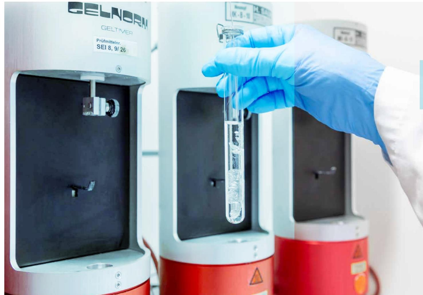
Measuring gel time: the reactivity of WACKER silicone resins is measured in a lab. Measurement curves can be found on page 24.
