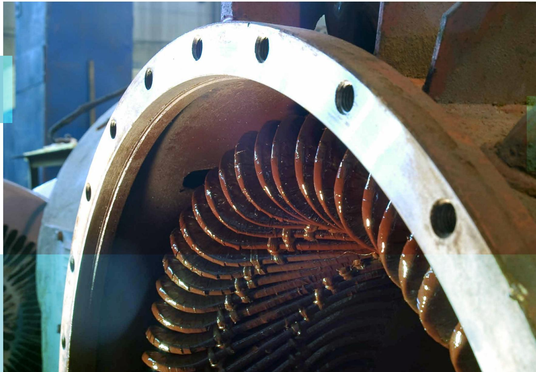
Preformed coils for electric motors of railway vehicles: such large stators are impregnated with SILRES® H62 C by vacuum-pressure impregnation.
