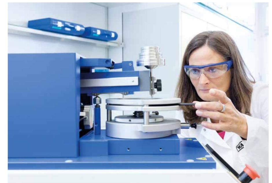
In the Erichsen scratch test, a needle moves at a specific force and speed across the plastic being tested, creating a grid pattern of scratches. The scratches are then examined closely and the color differences determined with a colorimeter.
