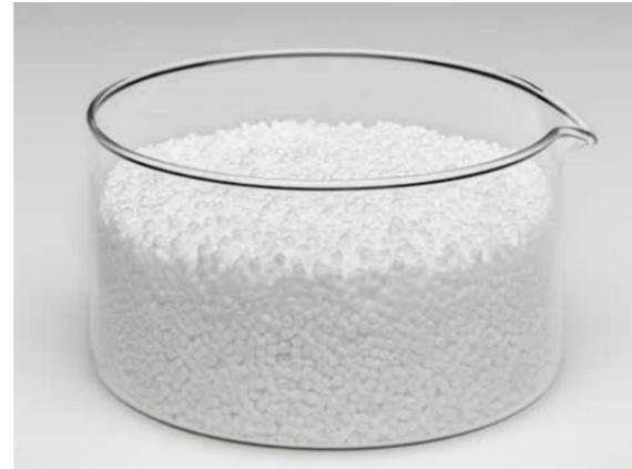
Silicone additives – here as ready-to-use pellets – facilitate the production of workable polyethylene molding compounds and improve the surface properties of the resulting plastic articles.
