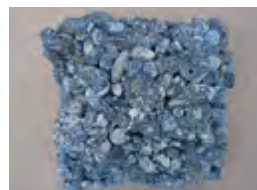
Without ETONIS®: >2,500g/m 2 (destroyed after 12 cycles)
