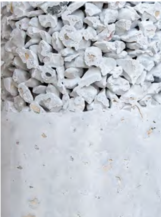
Dense and stable: Self-filling concrete fills in the gaps between the stones in the bottom half of this example.
