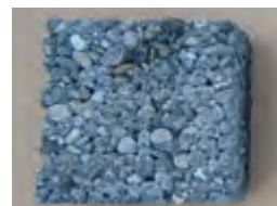
With ETONIS®: 880g/m 2 (28 cycles passed)
