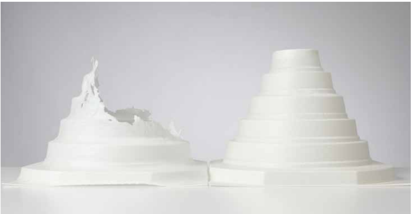
Compared to a regular PBS/PLA blend with chalk (picture on the left), the addition of VINNEX® powder enables proper thermoforming (picture on the right).
