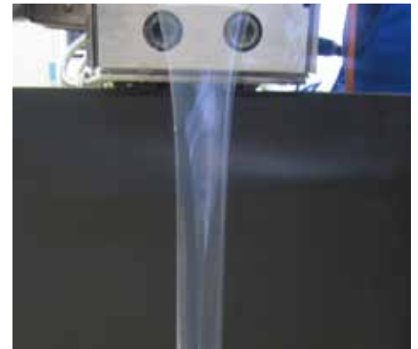
Compared to pure PLA (top image) the PLA/VINNEX® 2525 blend (bottom image) exhibits improved melt strength.
