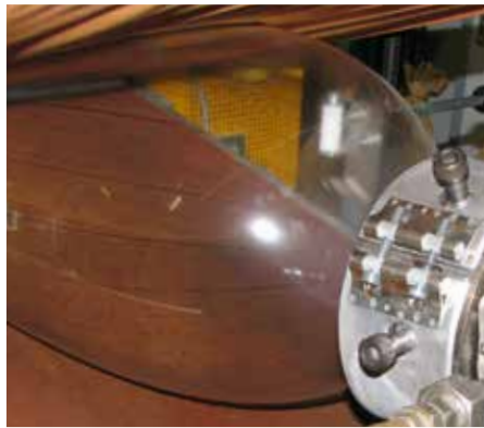
PLA/VINNEX® 8880 blend in blow film extrusion for highly transparent films.
