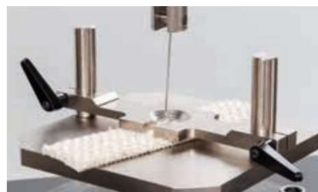
The tuft bind test examines how well the precoat adheres the fibers to the primary backing.
