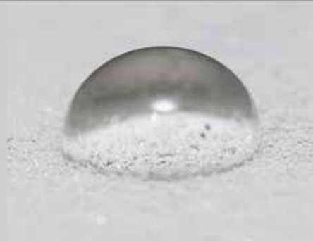
Water droplet on a dirty silicone surface.
