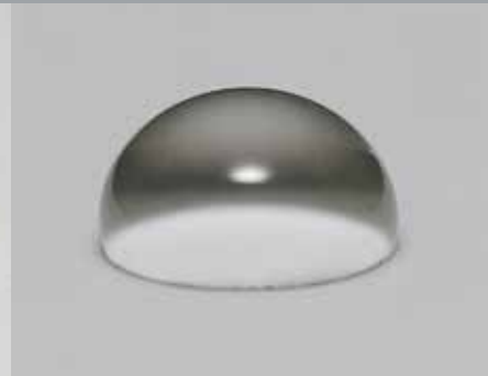
Water droplet on a clean silicone coating.
