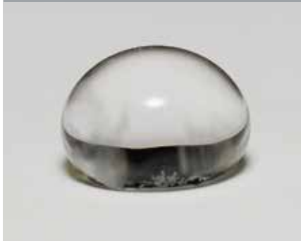
Water droplet on a dirty silicone coating.
