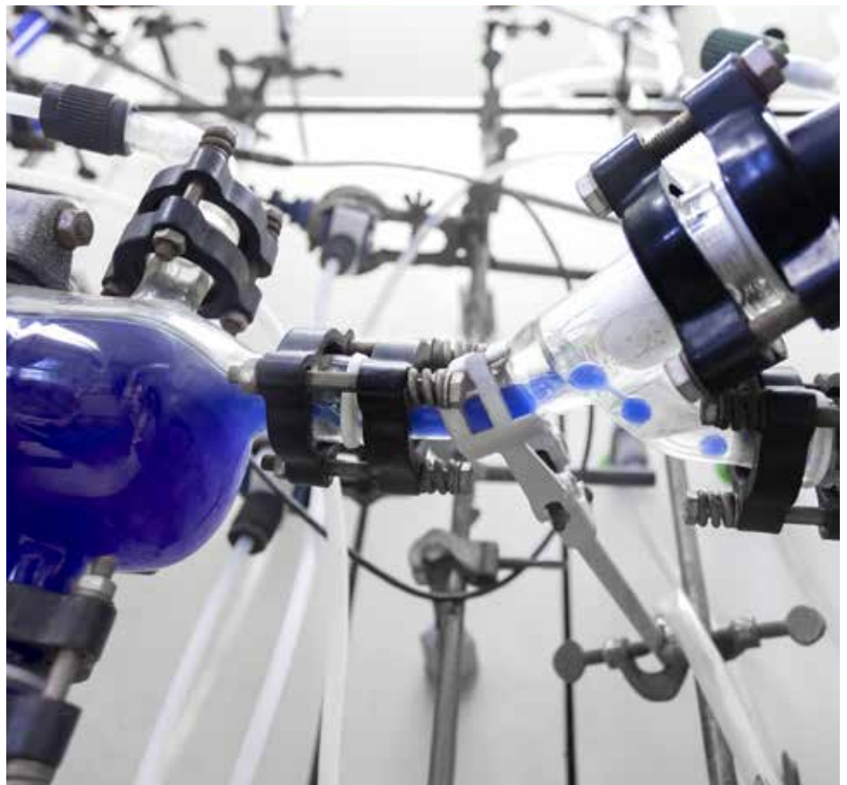
Loop reactor in WACKER's Technical Center for resins
