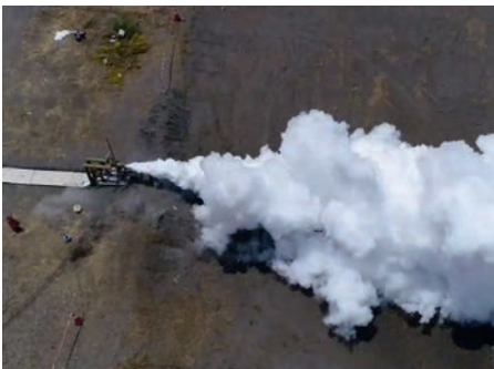
Release test at the Plataforma Solar de Almería (PSA) performed in May 2018 by CIEMAT (Centro de Investigaciones Energéticas, Medioambientales y Tecnológicas), DLR and TÜV-Nord (TÜV-report) showed no self-ignition of HELISOL® 5A.
