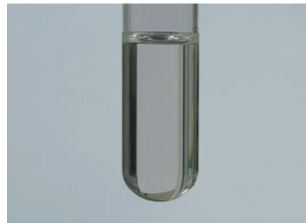
HELISOL® heat transfer fluids operated at 425 °C
