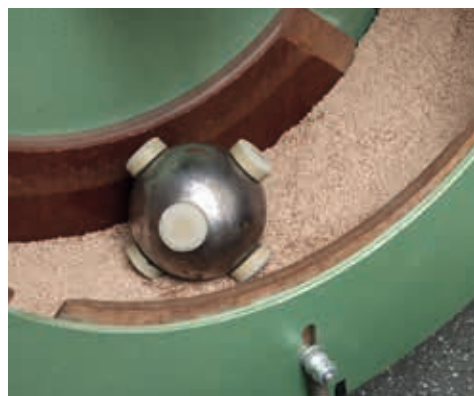
The Vettermann Drum test mimics the daily stress which a carpet is submitted to. This is especially important for commercial carpet applications.
