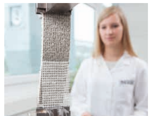
The delamination test evaluates the adhesion of the secondary backing to the carpet. This is mainly determined by the secondary coating.
