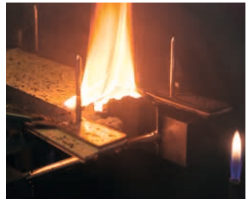
SB latex/calcium carbonate film (150% filler loading) according to DIN 4102-1.
