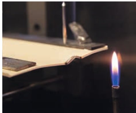
VAE/calcium carbonate film (150% filler loading) according to DIN 4102-1; self extinguishing.
