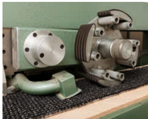
The Lisson test resembles the strain of shoes on carpet – this way the durability of the carpet can be tested.
