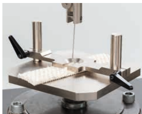
The tuft bind test examines how well the precoat adheres the fibers to the primary backing.
