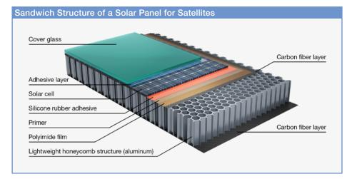
WACKER® RTV-S 691 can be applied by any conventional coating method such as dispensing, knife coating, transfer roller coating, screen printing, etc.
