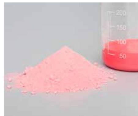
NEXIVA® based powder paints are simply mixed with water to produce a liquid paint. Paint preparation is easy and can take place either at the manufacturer's, at a sales location or on the job site.
