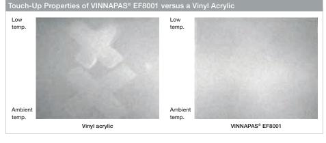
VINNAPAS® EF8001 exhibits excellent ambient- and low-temperature touch-up properties, even when formulated at low VOC levels.
