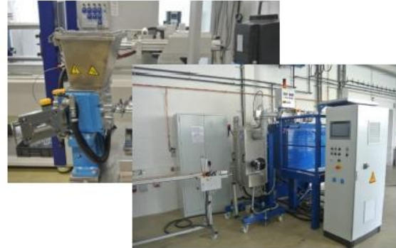
Compounding and extrusion of high consistency silicone rubber (HCR)
