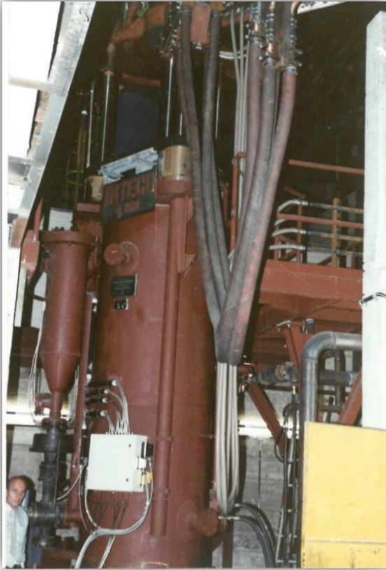
Pressurized (42 bar) ESR at Krupp Schmiedewerke Essen, Germany, 1980
