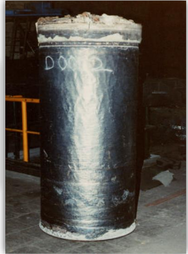
800mm dia. (8ton) ingot produced @ 42 bar
