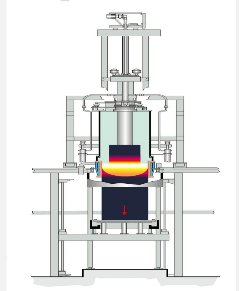
Retractable Mold Design with electrode exchange (semi enclosure system) and ingot withdrawal
