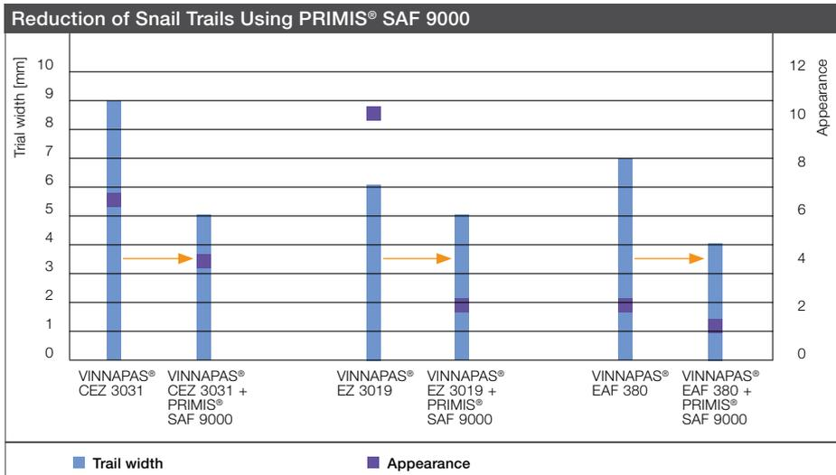
The graph shows the effect of PRIMIS® SAF 9000 as a co-binder in different formulations (proportion of binders: 80/20; facade paint with 4% blue pigment) after 14 days' curing. The appearance is assessed on a scale from 0 to 12. The lower the value the better the appearance. As for measuring the snail-trail width, the lower the number the better.
