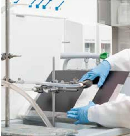
PRIMIS® KT 3000 is tested by applying a sample to a glass plate and storing it in a climatic chamber for six hours at 5 °C and 85% humidity. The sample is then exposed to simulated heavy rain for 20 minutes.
