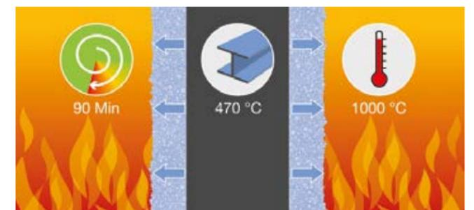
Figure 2: steel column with intumescent coating
