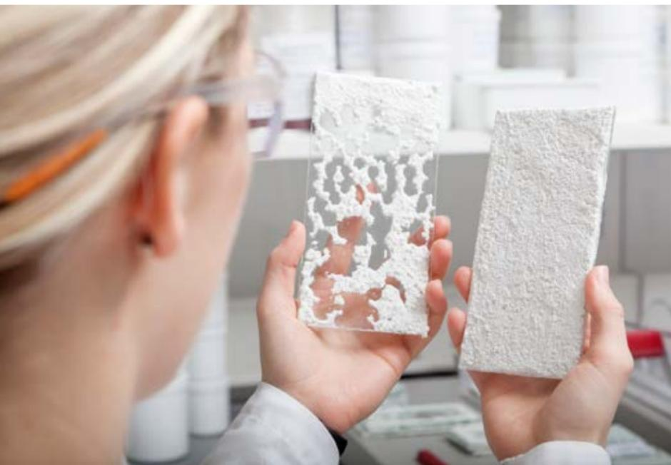
Direct comparison in the laboratory: after six hours' drying time, the test surfaces are irrigated. While the commercial plaster (left) does not withstand the moisture, the plaster modified with PRIMIS® KT 3000 (right) has formed a stable polymer network after only a few hours.
