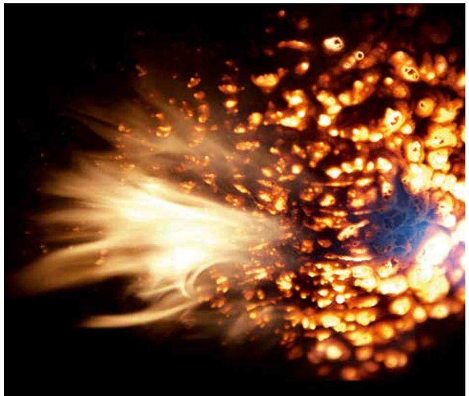
Fire test with a model intumescent coating formulation containing VINNAPAS® binders
