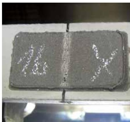
Testing the crack-bridging ability in accordance with EN 14891 at a WACKER technical center.
